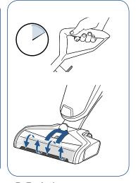
5. Each time you use the product, hold the solution trigger for 10 seconds to prime the system with cleaning solution before you begin cleaning. When you pull the trigger, LED lights will illuminate.
