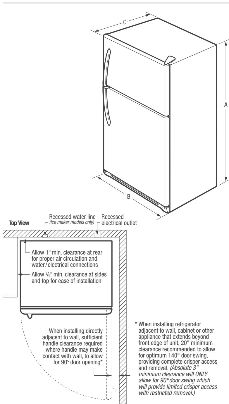
\* When installing refrigerator adjacent to wall, cabinet or other appliance that extends beyond front edge of unit, 20" minimum clearance recommended to allow for optimum 140° door swing, providing complete crisper access and removal. (Absolute 3" minimum clearance will ONLY allow for 90° door swing which will provide limited crisper access with restricted removal.)
