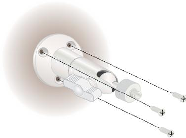
If you're mounting the camera on drywall, use the drywall anchors we provide.
