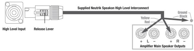
• For Differential (i.e. fully balanced) amplifiers using one REL, simply use the standard connecting scheme above. Connect the black wire to a ground lug or chassis screw. Should hum occur using this method, the black wire should be allowed to "float" or hang down without connection to ANY terminal.
