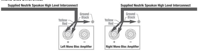
• If connecting a single REL as a dedicated centre channel sub, twist together the red and yellow wires and connect these paired wires (red/yellow paired together) to the positive centre channel amplifier terminal. Connect the black wire to a ground lug or chassis screw on the amplifier.
