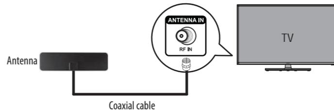
• **Digital converter box or set-top box:** Connect the coaxial cable to your digital converter box or set-top box, then connect a video/audio cable (such as an HDMI, coaxial, or AV cable) from your converter box or set-top box to your TV.
